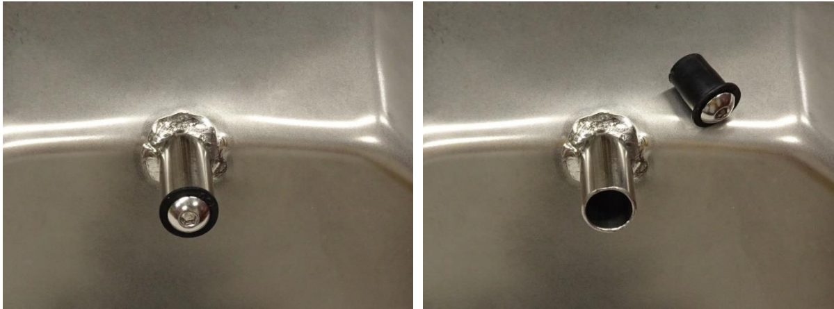
Figure 6. Drip tray upside down showing the plug left and plug removed right.
