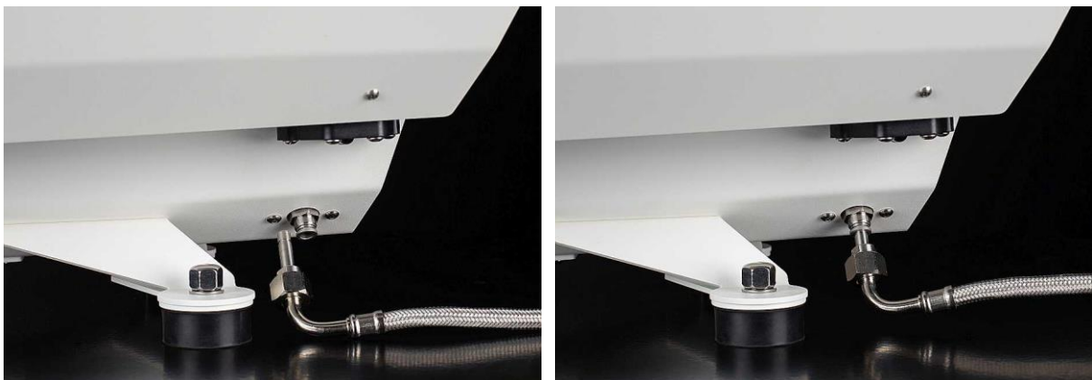
Figure 5. \varnothing=8\text{mm} push-in water mains connection at the back right of the machine and reinforced hose with push-in adapter.
